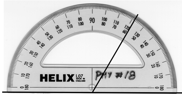
Wrong The angle is not 58° Figure 2
